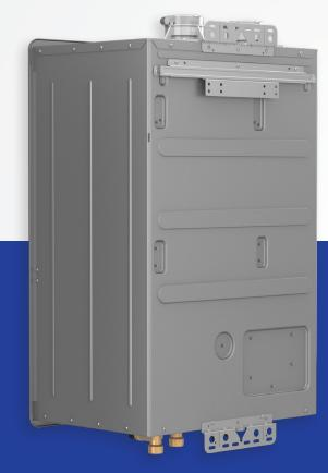
Friedrich® SR-Series can be installed either with direct vent (outside air) or non-direct vent (room air) intake. Room air intake allows maximum installation flexibility in an open area like a basement or garage, as well as in smaller spaces like a closet with full louvered door.
