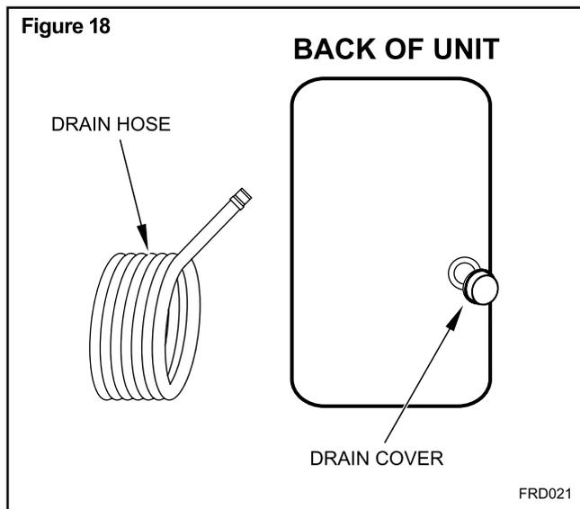
Unscrew and remove the drain cover at the rear of the unit (See Figure 19). Remove the soft rubber stopper. Put it into the drain bucket for safe keeping (See Figure 19).
