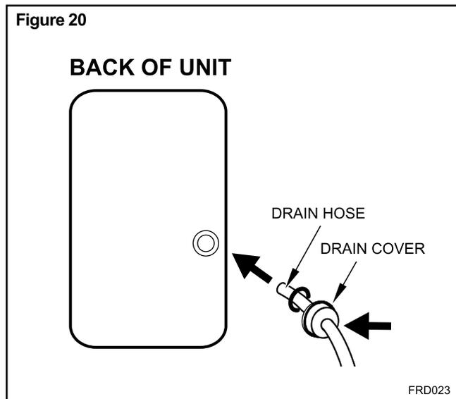
Tighten the drain cover in clockwise direction onto the rear of the unit (See Figure 21).
