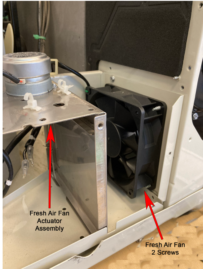
Figure 528 (Remove Fresh Air Actuator and Fan)
