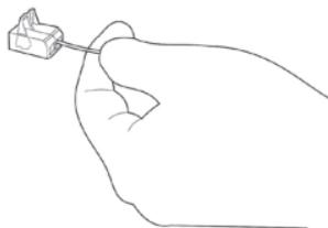
3. Insert the twisted wires from the CAT6 cable into the remaining lever connector slot as shown in Figure 4. Each twisted, paired wire should be inserted into its own separate slot in the lever connector.
