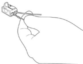
4. Close the orange lever on the lever connector as shown in Figure 5. Make sure the levers seat properly.
